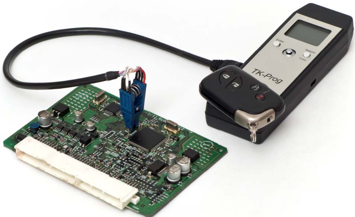
Fig. 7 Basic programming tool with smart-key on it
