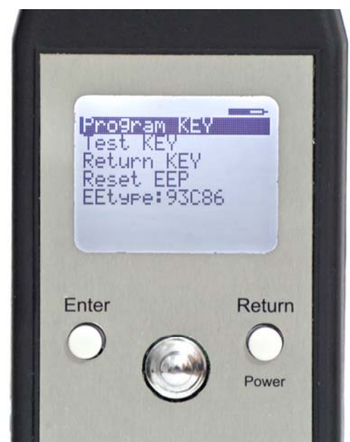
Fig. 3 Basic programming tool on-screen menu and navigation buttons
