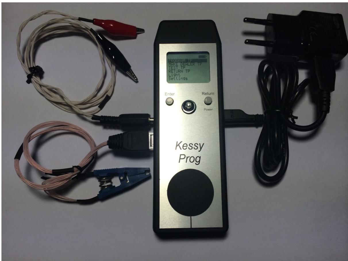
**Pic.1 Kessy Prog device with cables.**
